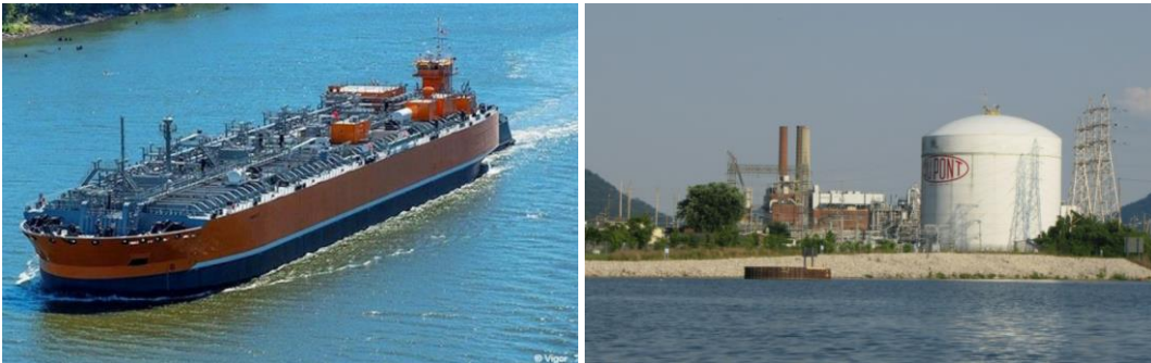
Figure 10-1: (left) example of 20,000 ton liquified ammonia barge (right) example of a 20,000 tonnes ammonia storage tank
