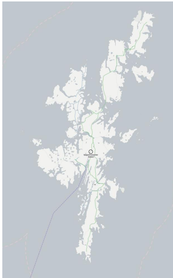
Figure 5-1: Map showing the HVDC interconnector (purple), 33kV lines (green) and 11kV lines (blue) [37]
