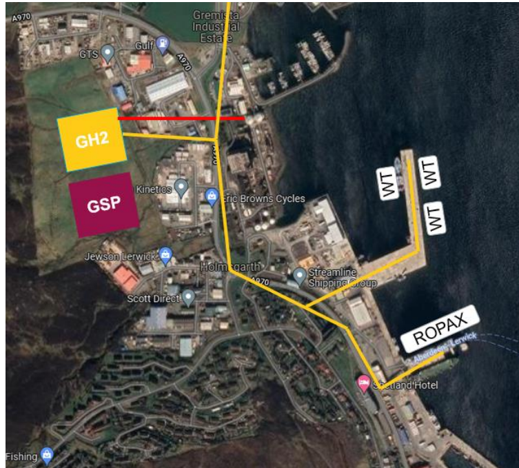
Figure 7-2 Grid supply point, electrolyser and pipework (yellow – hydrogen, red – waste heat to local heat storage)
